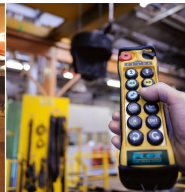
Flex 12EX system used on semi automatic crane with electrically operated grab
